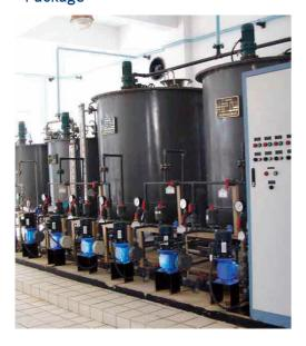
SC45 conductivity controller can be used together with the metering pump as a close-loop control system to improve water quality through controlling the liquid conductivity to reduce the content of metal ions in the solution, and it is widely used in circulating water treatment system.
